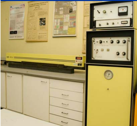
CO 2 laser pumped FIR laser \lambda up to 300 \mu\text{m}
