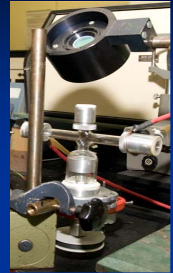
Laser ablation induced fast pulse discharge
