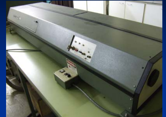
Nd:YAG laser 100 mJ 30 ns 10 Hz
